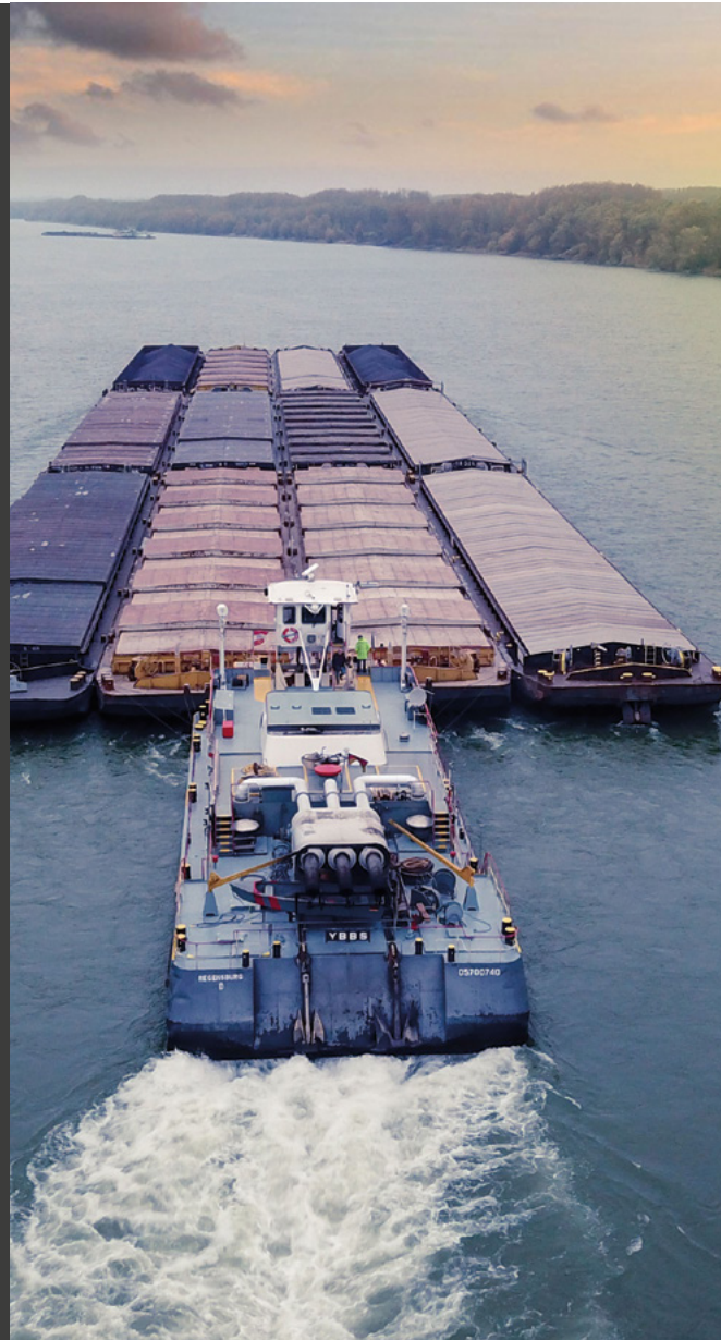
Image: First-DDSG vessel pushing 12 barges, carrying iron ore pellets at kilometre 285 of the River Danube.
